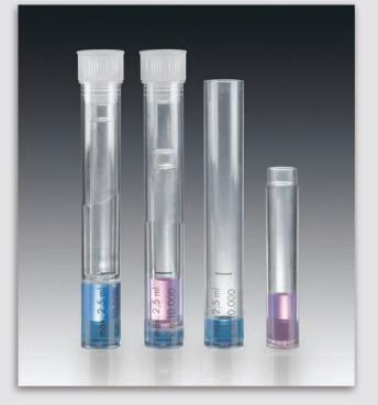
Centrisart<sup>®</sup> I ultrafiltration concentrators are disposable devices for biological samples. Centrisart<sup>®</sup> I is suitable for sample volumes up to 2.5 ml. The unique design allows ultrafiltration to take place in the opposite direction to the centrifugal force. This minimizes membrane blockage even with whole blood or cell lysate samples. The filtrate is collected in the floater insert tube where it is easily withdrawn.
