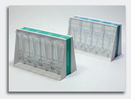
BJP concentrators offer fast and convenient means to concentrate antibodies and other proteins in research labs. This is done without a centrifuge, pressure or vacuum source. Absorbent pads pull solvent and microsolute through the ultrafilter concentrating the sample. A dead stop pocket at the bottom of each cell minimizes the chance to concentrate the sample to dryness. These BJP products are designed for general laboratory use and are available as individual units or as 8 test blocks.
